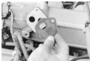
Fig. Fig. 6: When installing the valve, always discard the old gasket and install it using a new one
