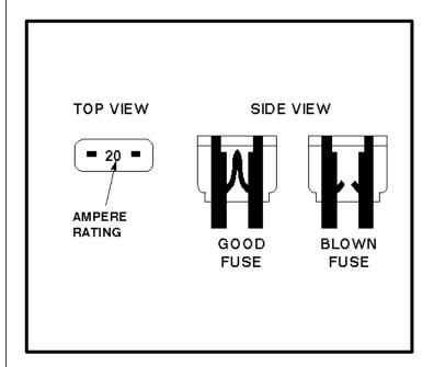
Blade type fuses have a transparent plastic housing. To check a fuse, pull it from the fuse panel and look at the fuse element through the housing. Always replace a blown fuse with a new fuse that has the same ampere rating.
