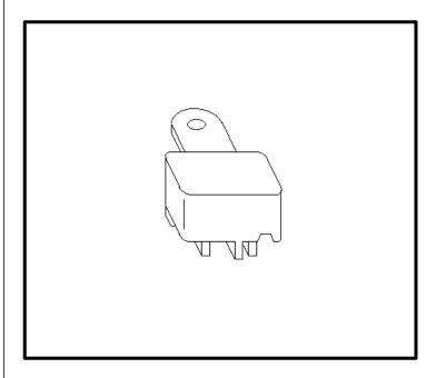
In the cycling type, the bimetal arm cools and straightens out. The cycle repeats as long as the overcurrent exists and power is applied.
