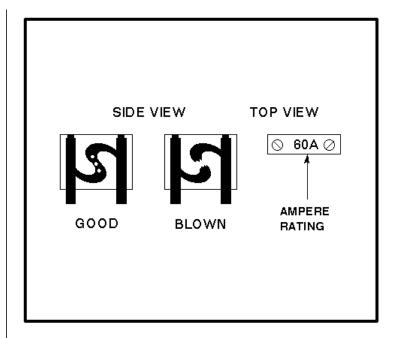
Maxi-fuse cartridges have a transparent colored plastic housing. To check a maxi-fuse, look at the fuse element through the top of the housing.
