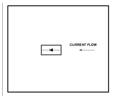
Diodes are electrical devices that permit current to flow in one direction only. The current flows in the direction indicated by the arrow.
