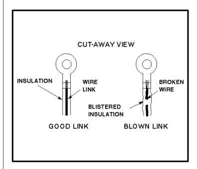
Fusible links are short lengths of wire that are smaller in diameter than the wires they are protecting. Fusible link wire is covered with a special thick, non-flammable insulation. An overload condition causes the insulation to blister. If the overload condition continues, the wire link will melt. To check a fusible link, look for blistered insulation. If the insulation is okay, pull lightly on the wire; if the fuse link stretches, the wire has melted.
