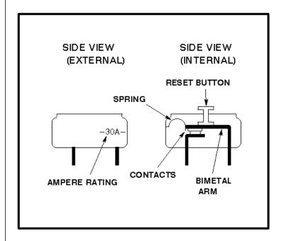
Two types of non-cycling circuit breakers are used; one is reset by removing power from the circuit, and the other is reset by depressing a reset button.
